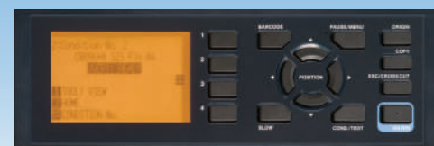
Intuitive 3.7" LCD Control Panel
